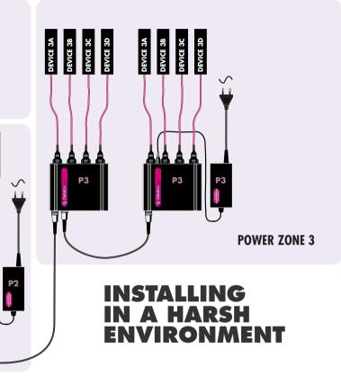
smartlink cables or TOUCHLINK units that are located away from the main rig, should receive power locally by means of 12V DC INJECTOR units, as indicated above for POWER ZONE 1.
